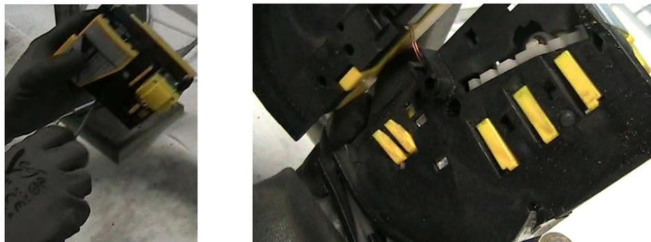
Remove dust and dirty particles from the optical sensor prisms. If matt or scratched, the prisms must be replaced.
